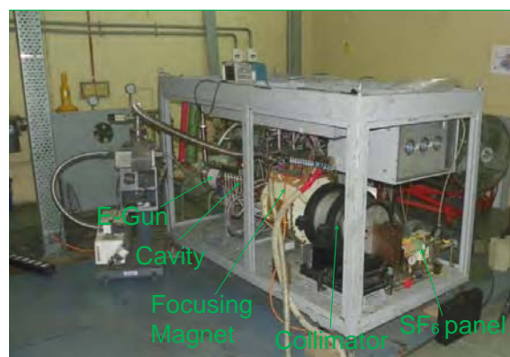
Fig. 1: 6 MeV compact linac.
