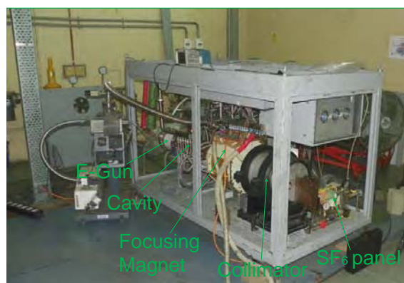
Fig. 1: 6 MeV compact linac.
