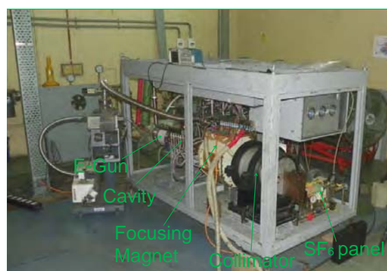
Fig. 1: 6 MeV compact linac.
