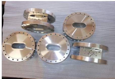
Fig. 5: A batch of 5 No. of laser welded SMA feedthrough BPIs after laboratory qualification.
