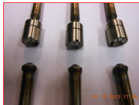
Fig. 2: Laser welded samples of location (1) broken by UTM.
