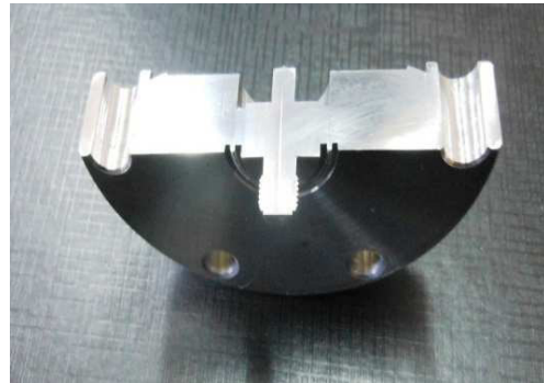
Fig.4:Etched sample of laser weld joint.
