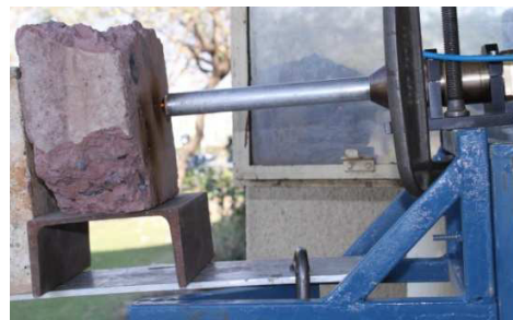
Fig. 2. A view of laser drilling of Hematite reinforced concrete.
