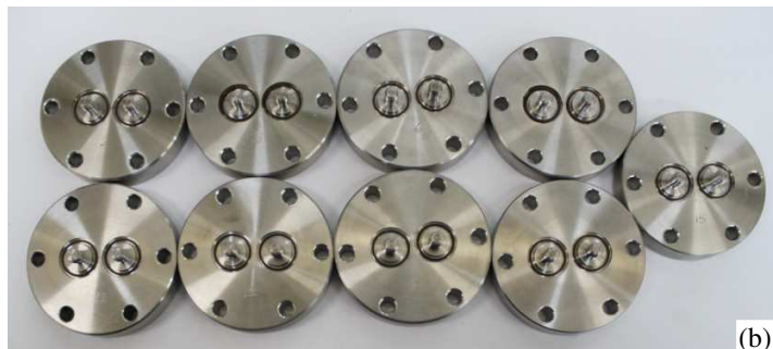
Fig. 5: (a) Nd:YAG laser welded sample of single SMA feedthrough, and (b) double SMA feedthroughs on one flange with optimized laser parameters.
