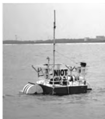
Wave energy buoy-BBDB during sea trial
