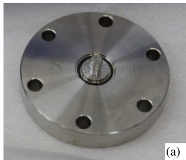
Fig. 5: (a) Nd:YAG laser welded sample of single SMA feedthrough, and (b) double SMA feedthroughs on one flange with optimized laser parameters.
